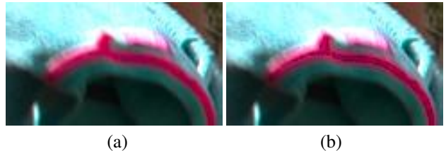
Fig. 1: Example of artifacts generated by chroma subsampling. (a) 4:4:4 full chroma sampling, (b) 4:2:0 MPEG chroma sampling.
